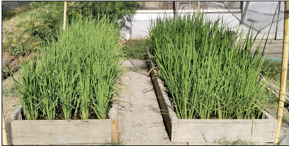
Figure 2. Experimental set-up using wooden box contains contaminated soil with cadmium
